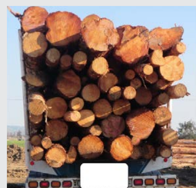
A top-heavy load. Bigger heavier logs loaded up high causing pins to splay.
